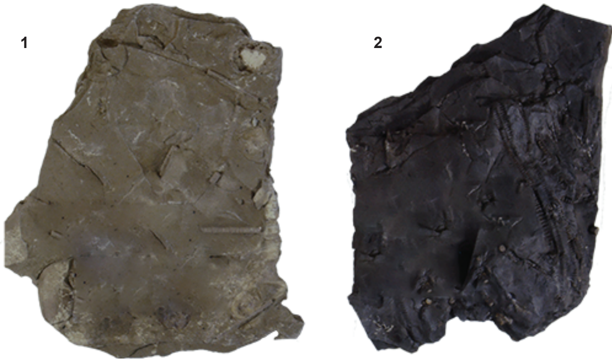
Text-fig. 2. Upper Ordovician (Katian Stage) marine mudstone samples containing nearly identical total organic carbon (TOC) levels, but displaying dramatic thermal maturity contrasts and appearance. Specimens collected at nearly opposite ends of Lake Ontario. 1 , Crinoid stem-bearing mudstone from the thermally immature lower part of Georgian Bay Formation collected along the Humber River, west of Toronto, Ontario, Canada, 43.663039, -79.506514 (5YR 5/1, TOC = 0.1%). 2 , Crinoid stem-bearing shale parting within the overmature Pulaski Formation, collected along the Salmon River at Pulaski in north-central New York State. Richland 7.5' quadrangle at ~43.555531, -76.105709 (N3.5, TOC = 0.2%). Samples submitted as part of new Paleontological Research Institution Mudstone Thermal Maturity Collection. Temporary sample numbers PRI 2826 (1), PRI 2801 (2).
